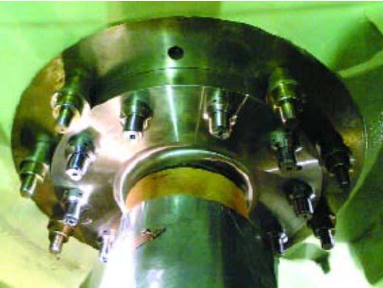
VLCC with ABS Classification installed with Pilgrim Radial Fit Bolts at the engine to 1st intermediate coupling flange
