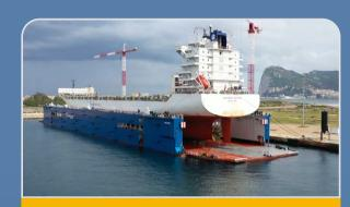
NEW FLOATING DOCK **230**x**39 m** LIFTING CAPACITY: **35.000**
