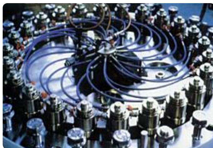
*Central feed individual tensioner simultaneous tightening*
