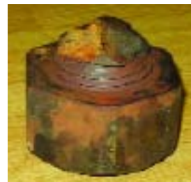
Damaged shrink fit bolt after removal
