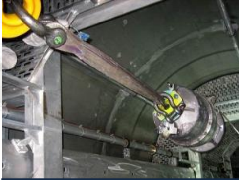
Cargo pump removal & overhauling
