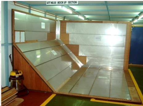
Invar Protection Mockup for GTT No. 88 , 96
